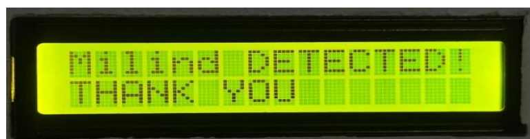
Figure 8: Display of Detected Message of theTrainedFace on theLCDScreen.
